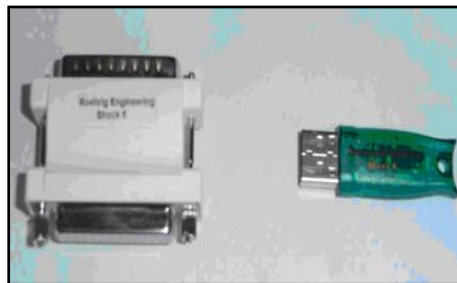
Figure #2: Software key – Parallel (old) and USB (Shock 6 and up)
